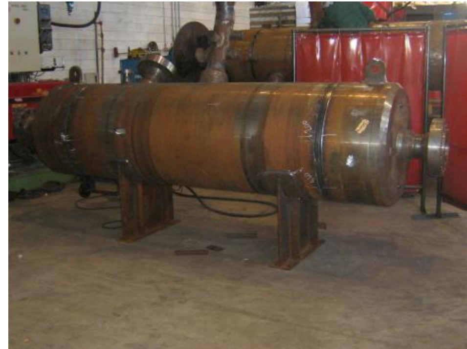
Volume bottles \varnothing 0,740 x 4,5 m - Thickness 68 mm
