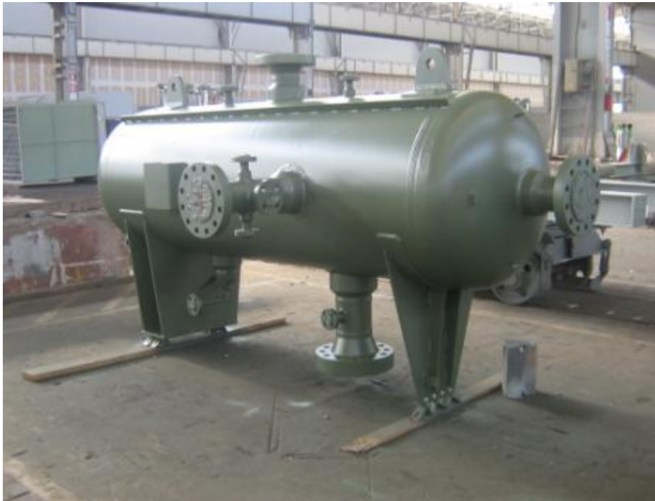
Bottles volume \varnothing 0,940 x 4,2 m - Thickness 45 mm
