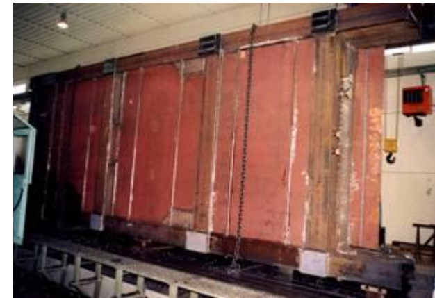
Gas Turbine Baseplate 3,6 x 10m x 13T GE OIL&GAS - Florence (Italy)
