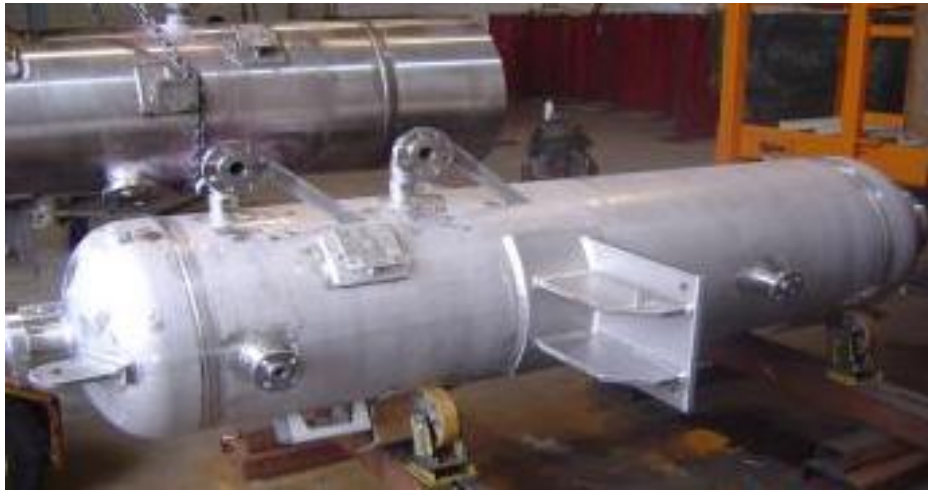
Pressure Vessel in AIS 304 SS Ø 0,7 x 3,6m x 60mm - 140 bar Ammonia/Urea Plant UDHE – Damietta (Egypt)
