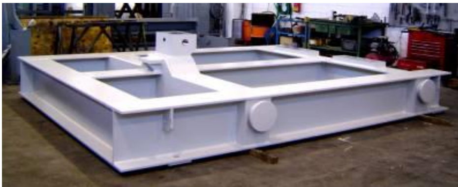
Transport Baseplate for a gas turbine 3,3 x 4,2m GE OIL&GAS - Florence (Italy)
