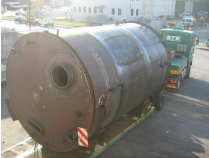
Hydrocarbon Liquid Condensate Tank Ø 3.660 mm H=5.800 mm
