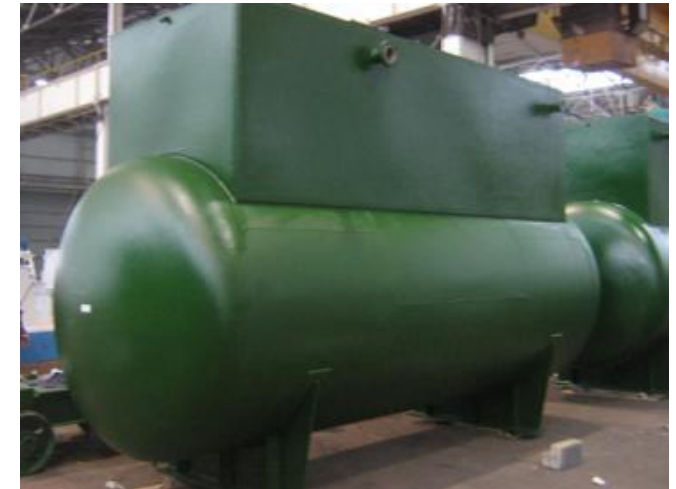
Fuel Oil Buried Tank Ø 1.750 mm L=5.410 mm
