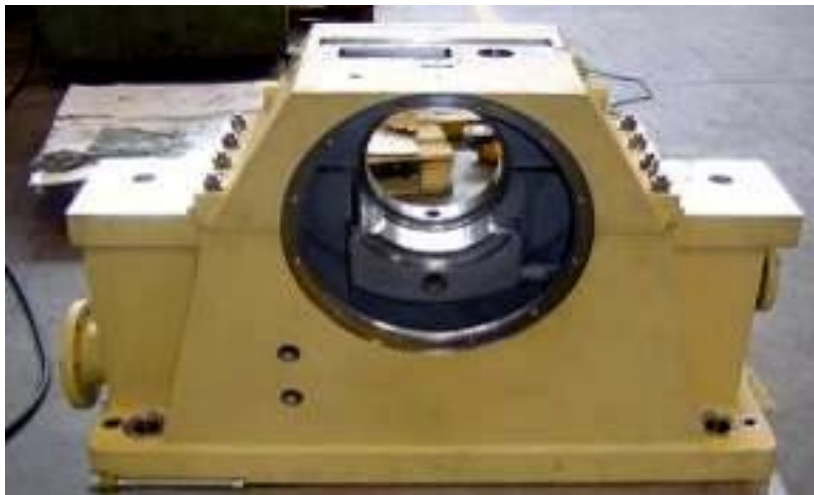
Steam turbine Bearing Boxes 1,5 x 2,5 x 1,5m x 8T GE OIL&GAS - Florence (Italy)
