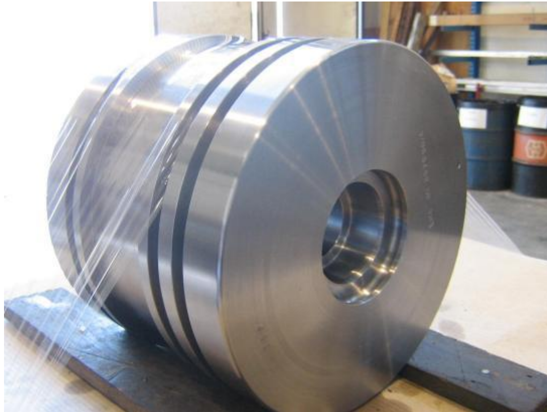
Piston in welded steel for Reciprocating Compressors GE OIL&GAS - Florence (Italy)
