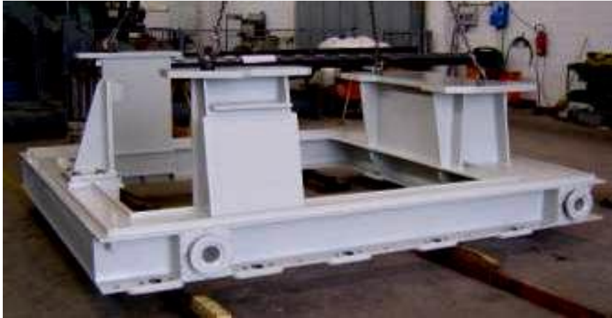
Steam turbine baseplate 3 x 3,5m x 4T GE OIL&GAS - Florence (Italy)
