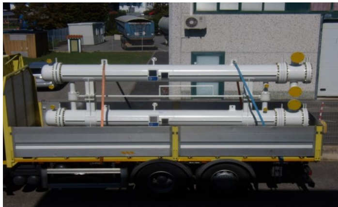
Nr. 6 alcohol production Heat Exchangers Ø 1,35 x 10 m AGRANA Bioethanol – Pischeldorf (Austria)
