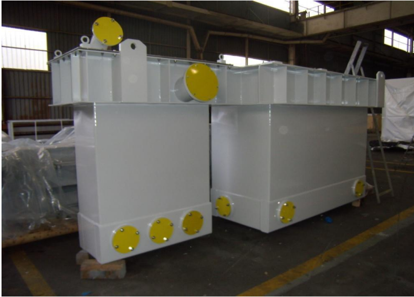
Nr. 8 Mineral Lube oil Console 4 x 3 x 2 m x 7,5T AISI SS 316L INPEX- HYTCHYS (Australia)
