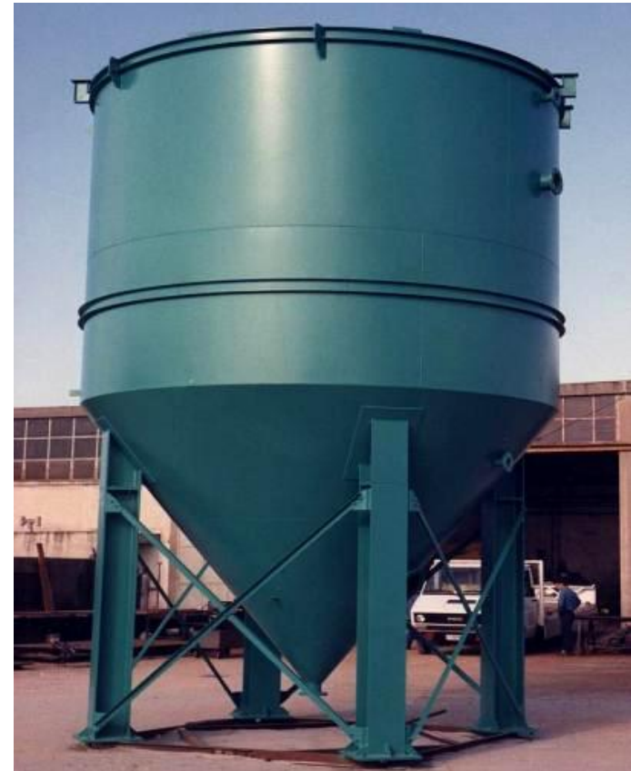
Water treatment silo (food grade) Ø 4 x 5m x 10T COCA COLA Livorno (Italy)
