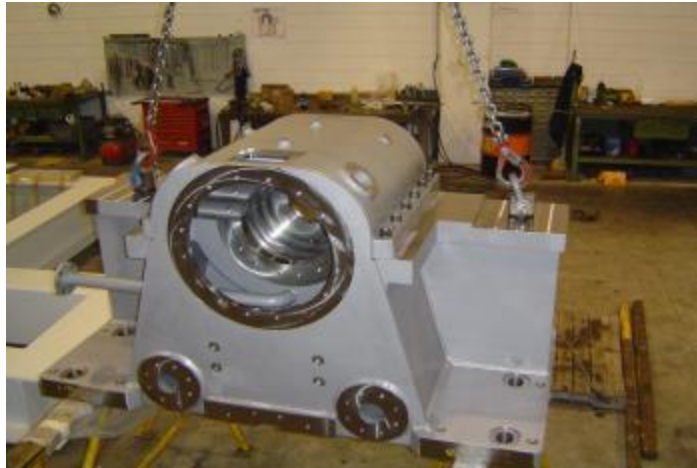
Steam turbine Bearing Boxes 1,5 x 2,5 x 1,5m x 8T GE OIL&GAS - Florence (Italy)
