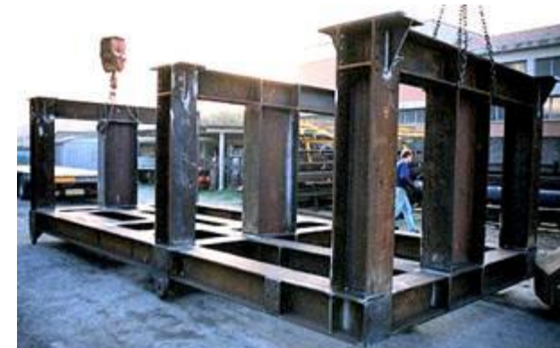
Gas Turbine Baseplate 3 x 2,5 x 10m x 11T GE OIL&GAS - Florence (Italy)
