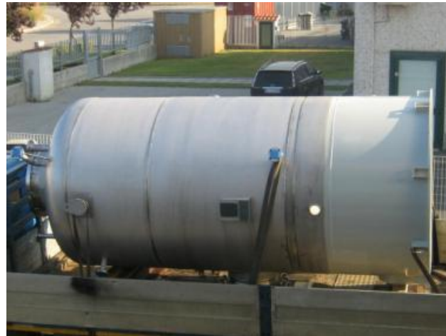
Liquid Sloop Tank (AISI 304) Ø 2.000 mm H=4.525 mm
